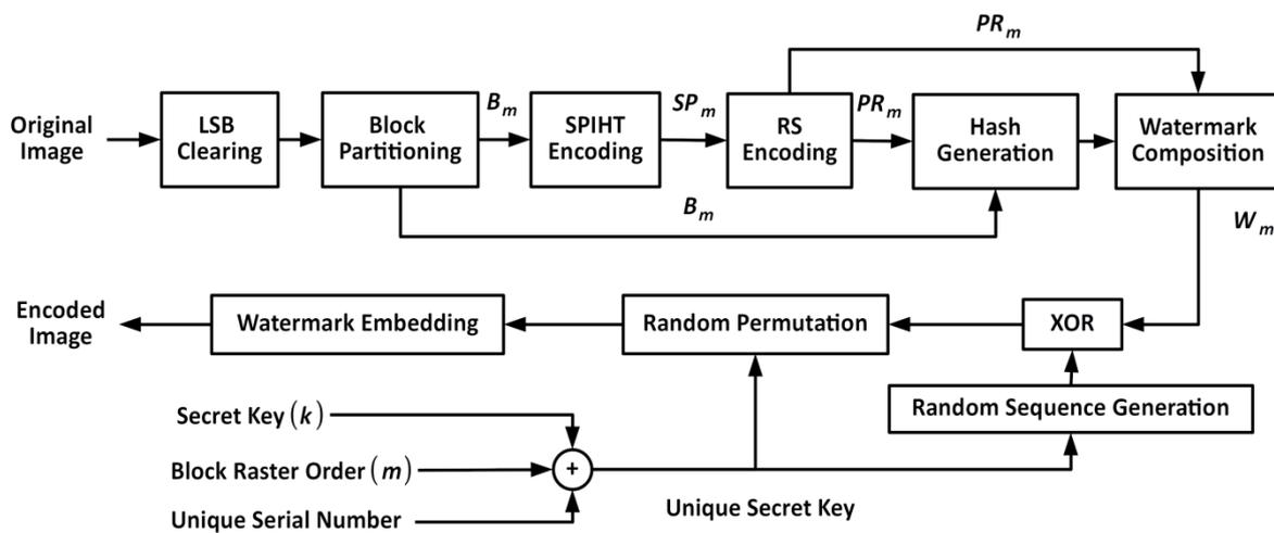
Fig. 1. Block diagram for the encoding stage of the proposed method.
