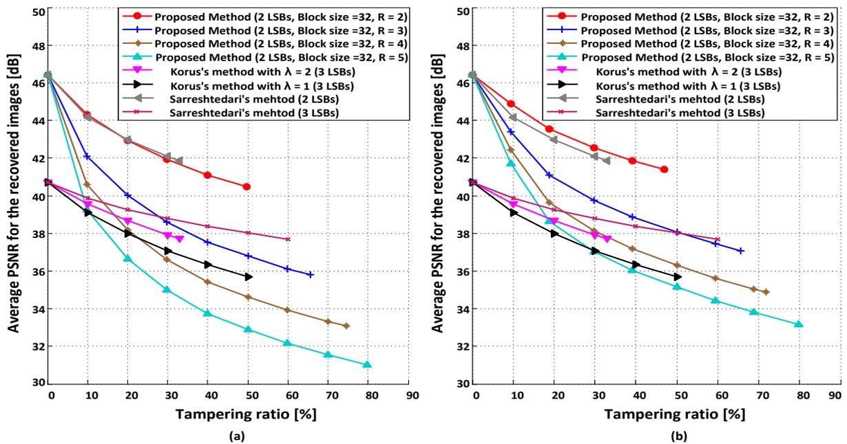
Fig. 4. A comparison between Sarreshtedari's, Korus's, and the proposed method, showing the average PSNR for 1000 images chosen from BOWS-2 data-set; block sizes in the proposed method are: a)  $32 \times 32$ ; b)  $64 \times 64$ .
