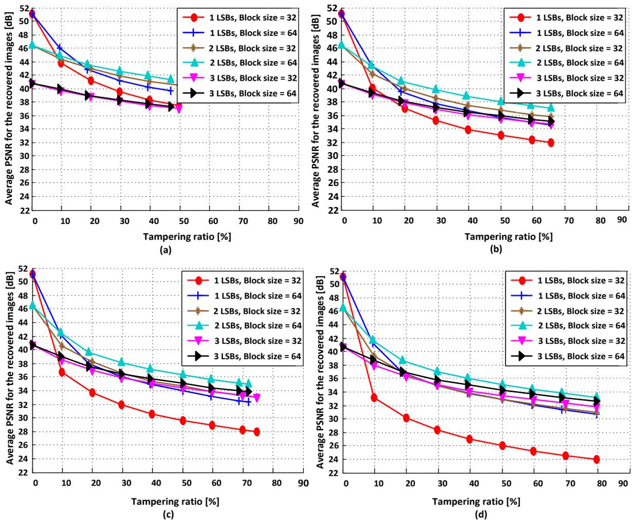
Fig. 3. Average PSNR for 1000 random images - chosen from BOWS-2 data-set - for code-rate reciprocal  $R$  values of: a) 2; b) 3; c) 4; d) 5.
