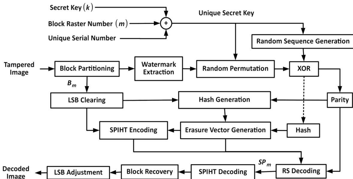
Fig. 2. Block diagram for the decoding stage of the proposed method.
